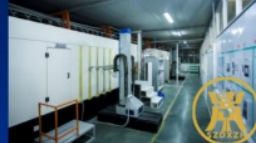
Reciprocating machine (automatic powder spraying)
