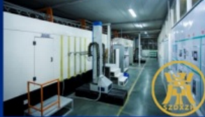
Reciprocating machine (automatic powder spraying)
