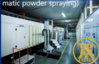
Reciprocating machine (automatic powder spraying)
